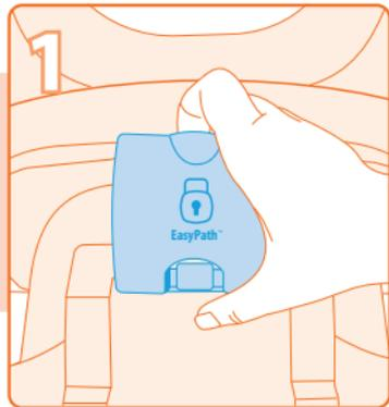
1. Find the EasyPath™ Belt Lock-Off and **open** the clamp by **pulling down** then **up** on the top tab.
