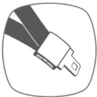
3. **Lap/Shoulder Belt with Locking Latch Plate.** The lap portion of this belt does not loosen once the belt is buckled.
