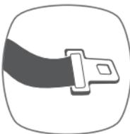
2. **Lap Belt with Automatic Locking Retractor (ALR).** The automatic locking retractor does not allow the lap belt to get longer once it is buckled and retractor is locked.
